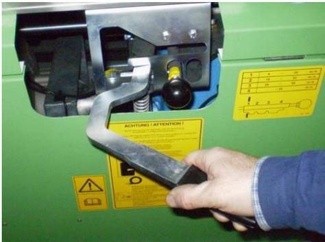
Move gear shift lever into the “PE-pipe pull-off” position. A spring presses the lever up and locks it.
