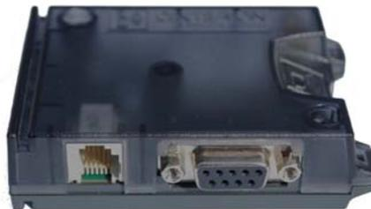
Das **BGS2T GSM Modem by Cinterion** has a LED showing status.
