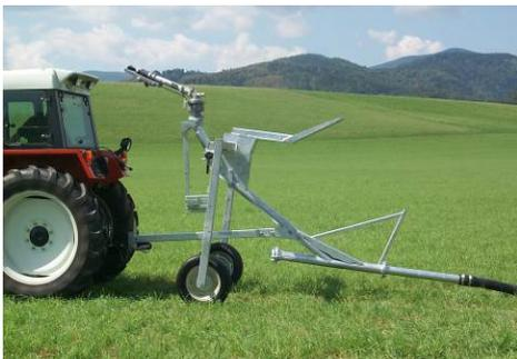
For easier PE-pipe pull-off the carts are equipped with a double draw-out hook. You pick up this hook with the tractor's toolbar and pull off the PE pipe.
