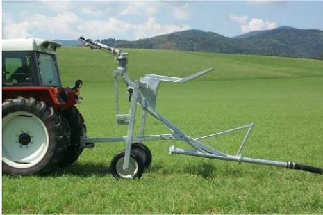
Pick up the double draw-out hook with the toolbar and pull the cart into the field.
