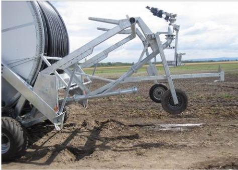
After retraction of the PE-pipe the machine supports can be carefully withdrawn with the tractor's hydraulic system. In doing so the cart is lifted into the transport position automatically.
