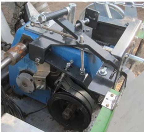
BAUER change-speed gearbox reduces the turbine speed according to the set turbine revs. The gearbox incorporates four gears. Reel drive stop at the end of the irrigation strip is ensured by disengagement of the tooth clutch.
