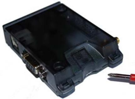
Connect communication-, power and antenna cable.
