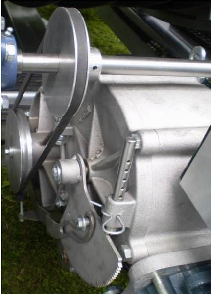
The full-flow turbine TVR 60 is a specifically designed model with large cross sections and minimum pressure loss. Therefore they are also suited for high retraction speeds at very low flow rates. These turbines feature a very flow-promoting design and they are mounted directly on the reel shaft. They provide the energy needed for the PE-pipe retraction. The turbine speed is taken directly off the impeller shaft and transmitted over a V-belt drive to the BAUER change-speed gearbox.
