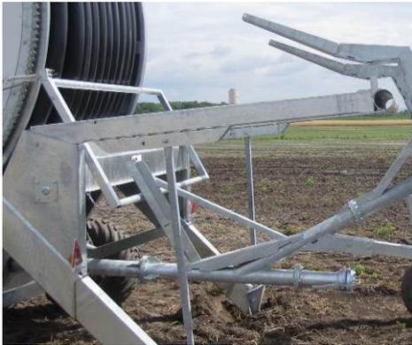
Unattended operation of the RAINSTAR is made possible by a final and safety shut-off. The final shut-off is actuated when the sprinkler cart pushes against the shut-off frame, which in turn operates the shut-off lever through a system of rods. This way the drive is stopped.
