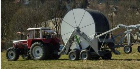
When transporting the machine, the cart has to be mounted to the lift frame in lifting position. The machine supports are fold up and the tractor jack is completely drawn-in.
