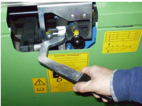
Shift the shut-off lever to the "PE-pipe pull-off" position.
