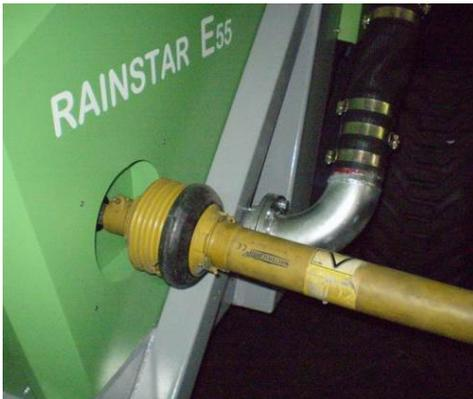
If required, you can rewind the PE-pipe also with the tractors PTO system
