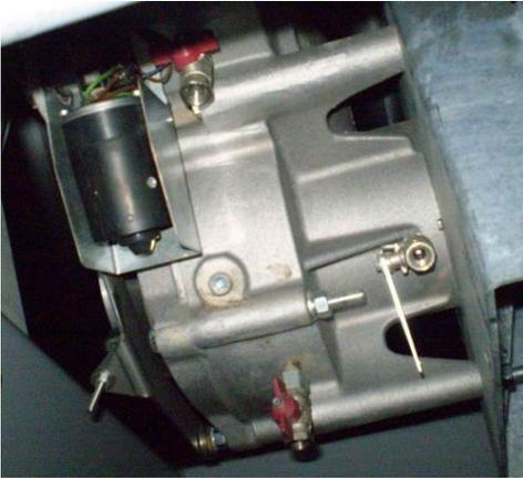
Open the drain valve on turbine
