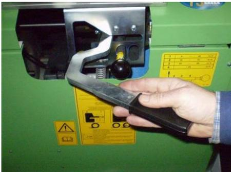
2. Pull the shut-off lever into the shut-off position and push it downward slowly and carefully...
