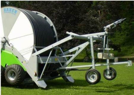
When the supports are being extended the cart is automatically lowered into the “PE-pipe pull-off” position.
