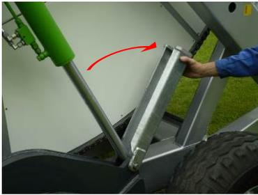
Unfold the locking device for cylinders till it touches the stop bar.
