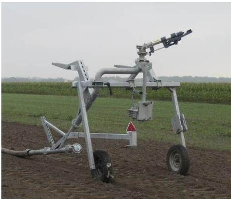
The high construction of both symmetric and asymmetric wheel carts provides maximum crop protection (Asymmetric wheel cart OPTIONAL). With infinitely variable track width the carts adapt to any crop row spacing. The width is symmetrically adjusted with the frame support member.
