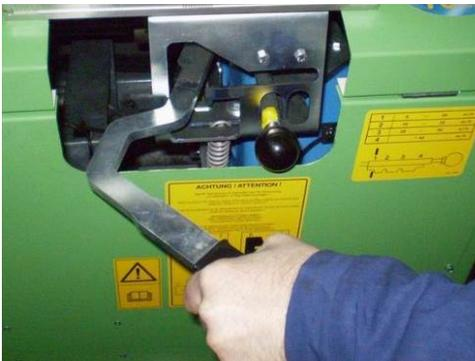
Slacken the PE-pipe by pushing down the gear shift lever carefully.
