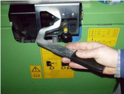
If something unforeseen happens, the pipe retraction can be interrupted with the emergency shut-off. Pull the gear shift lever with the open hand from the “PE-pipe retraction” position to the shut-off position (Do not operate the lever with the closed hand or release it immediately !). The gearbox is disengaged.
